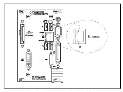
Figure 3-4. Ethernet Connector Location and Pinout
